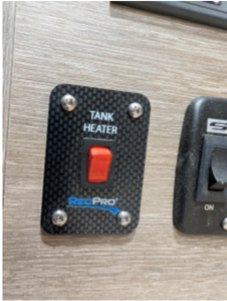
Heating Pad Switch
